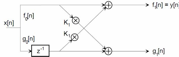
$$\begin{aligned} f_1[n] &= x[n] + K_1 x[n-1] \\ g_1[n] &= K_1 x[n] + x[n-1] \end{aligned}$$
