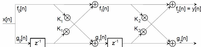
$$\begin{aligned} f_1[n] &= x[n] + K_1 x[n-1] \\ g_1[n] &= K_1 x[n] + x[n-1] \\ f_2[n] &= f_1[n] + K_2 g_1[n-1] \\ g_2[n] &= K_2 f_1[n] + g_1[n-1] \end{aligned} \quad \begin{aligned} \alpha_2[2] &= K_2, \quad \alpha_2[1] = K_1(1+K_2) \\ y[n] &= f_2[n] \rightarrow \\ K_1 &= \frac{\alpha_2[1]}{1+\alpha_2[2]}, \quad K_2 = \alpha_2[2] \end{aligned}$$
